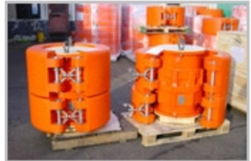
VIEW OF DOWNSTREAM SECTION OF BENTLEY STANDARD DOUBLE CLOSURE MARINE BREAKAWAY COUPLING FOLLOWING ACTIVATION AND RETRIEVAL OF FLOATING PIPELINE CONDUIT LIFT, SINGLE POINT MOORING TERMINAL, NOVOROSYISK, RUSSIA.
