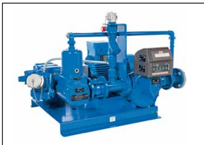
Mouvex Centrex metering unit for loading / off-loading of fuels with air eliminator
